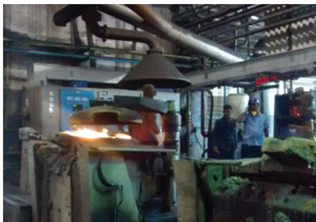
Figure 18: Induction furnace with lid mechanism
