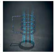
An induction heating system consists of an inductor (to generate the magnetic field) and a converter (to supply the inductor with a time-varying electrical current). Alternating current flowing through an electro-magnetic coil generates a magnetic field.
