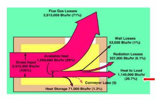
Figure 11: Sankey diagram of typical forging furnace
