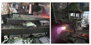
Figure 3: Conventional furnace oil fired forging furnace in Jalandhar hand-tool cluster
