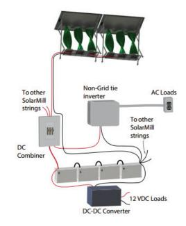
Figure 85: Hybrid mill connected to loads
