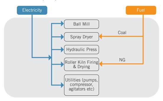
Figure 23: Ceramic tile manufacturing unit – Energy usage area
