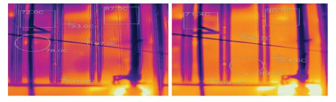
Figure 71: Thermal Image of Kiln
