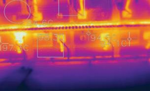
Figure 31: Thermal Image of Roller Kiln
