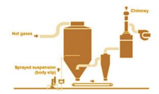
Figure 6: Spray drying process
