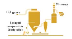
Figure 62: Spray dryer system
