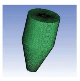
Figure 57: CFD Model of main drying chamber
