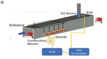
Figure 73: PID & VFD based excess air control system
