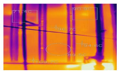
Figure 67: Surface temperature at firing zone in kiln
