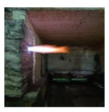
Figure 88: High Velocity Burner with Flame
