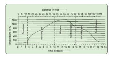
Figure 11: Firing cycle
