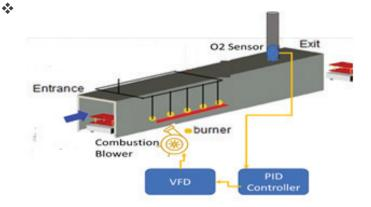
Figure 33: PID & VFD based excess air control system
