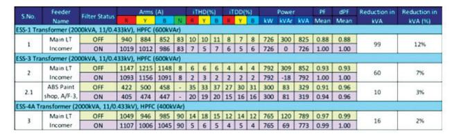
Figure 48: Reduction in kVA with & without operation of hybrid flter
