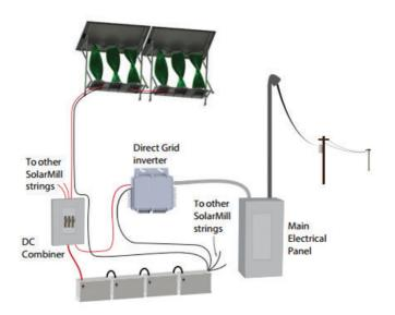
Figure 84: Hybrid mill connected to supply
