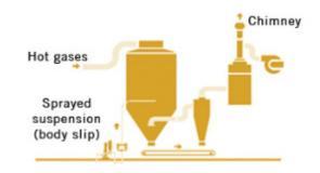
Figure 64: Spray dryer system
