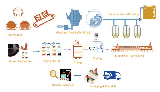
Figure 12: Ceramic pottery manufacturing process flow
