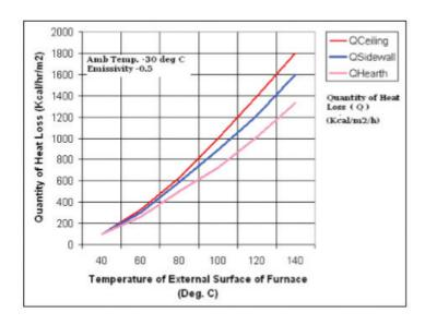
Figure 32: Quantity of heat loss from surface vs temperature
