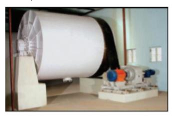
Figure 74: Conventional Ball Mill system
