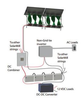
Figure 54: Hybrid mill connected to loads
