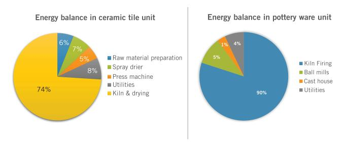
Figure 21: Energy balance in ceramic tile and pottery ware unit
