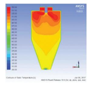
Figure 58: Contours of moister concentration and temperature distribution inside the chamber
