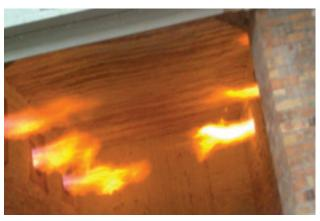
Figure 89: Perfect combustion with correct air fuel to ratio
