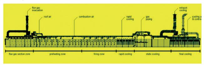
Figure 18: Tunnel kiln firing
