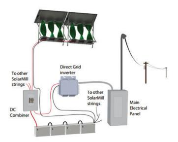
Figure 53: Hybrid mill connected to supply
