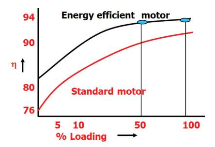
Figure 49: Percentage loading for Energy Efficient motors
