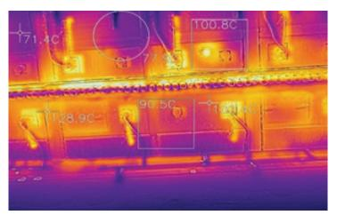
Figure 29: Surface temperature at firing zone in roller kiln
