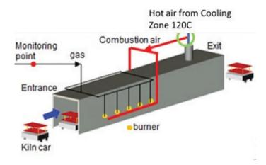
Figure 65: Implementation of WHR system in kiln – Use of hot air as combustion air
