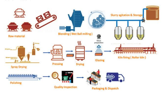
Figure 3: Ceramic tile manufacturing process flow
