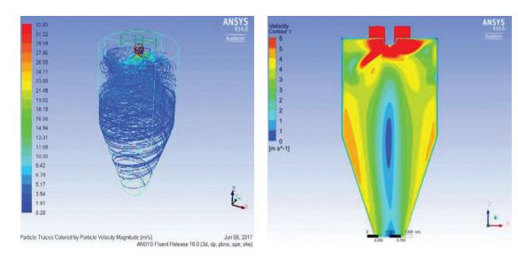
Figure 56: Particle flow pattern and velocity distribution inside the chamber
