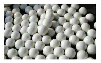
Figure 37: High Alumina Ball
