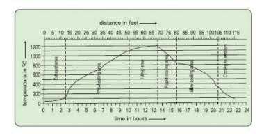
The kiln firing is done in two stages:
