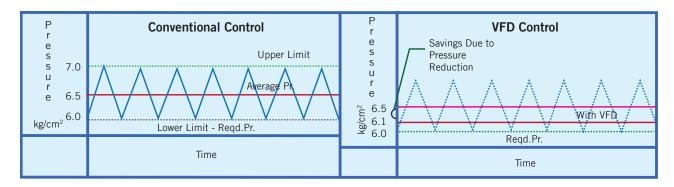
Figure 39: Capacity control of compressor
