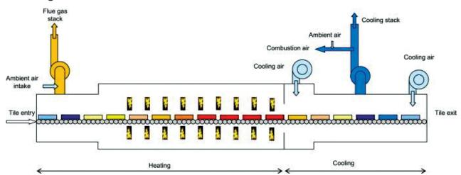
Figure 10: Tunnel Kiln firing
