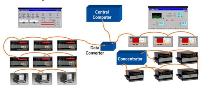
Figure 61: Components of Energy Management System
