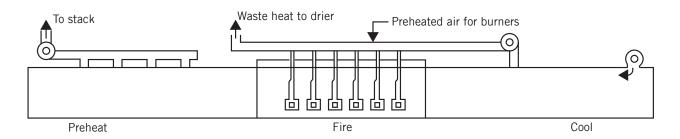
Figure 28: Zones in Roller Kiln
