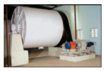
Figure 34: Conventional Ball Mill system
