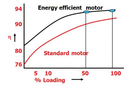
Figure 43: Percentage loading for energy efficient motors
