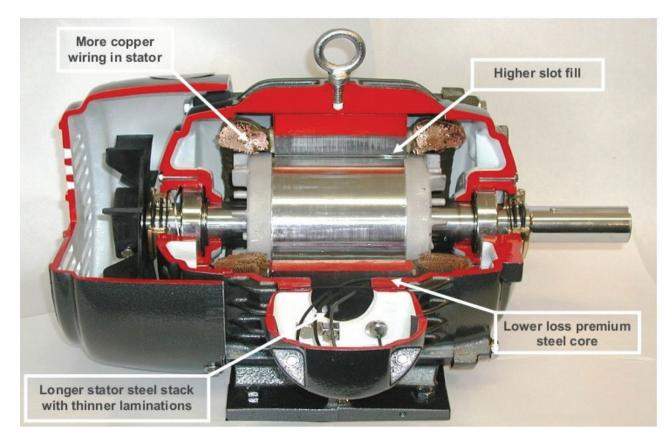
Figure 50: Energy Efficient Motors
