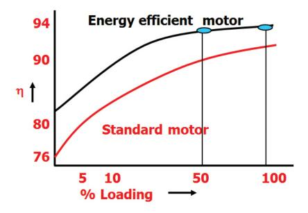
Figure 80: Percentage loading for energy efficient motor
