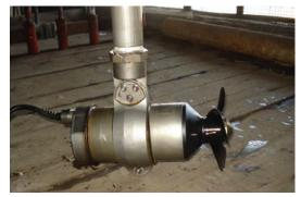
Figure 27: Submersible agitators
