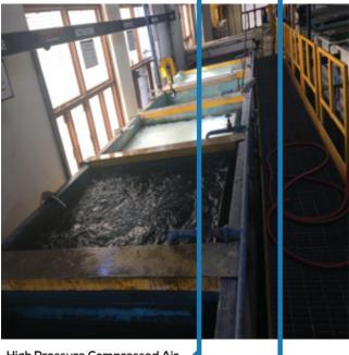
High Pressure Compressed Air Using @ 7 kg/cm<sup>2</sup> for Agitation
